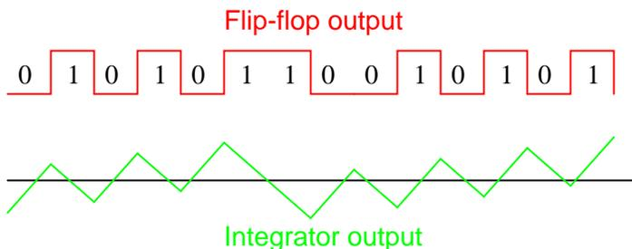
By applying a larger (negative) analog input signal to the integrator, we force its output to ramp more steeply in the positive direction. Thus, the feedback system has to output more 1's than before to bring the integrator output back to zero volts:
