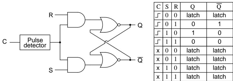
Only when the clock signal (C) is transitioning from low to high is the circuit responsive to the
