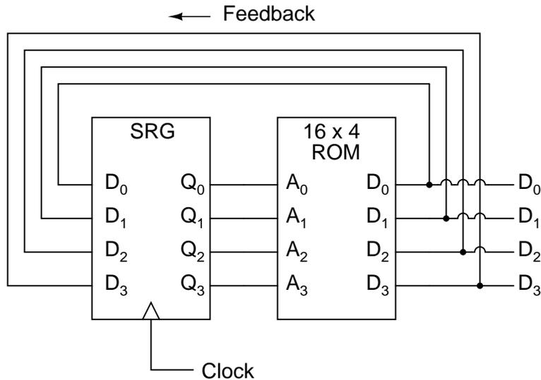
An analogy for the workings of such a device might be an array of post-office boxes, each one with an identifying number on the door (the address), and each one containing a piece of paper with the address of another P.O. box written on it (the data). A person, opening the first P.O. box, would find in it the address of the next P.O. box to open. By storing a particular pattern of addresses
