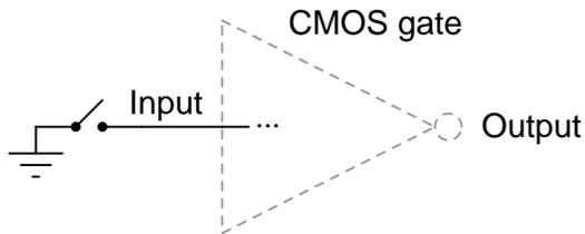
*When switch is closed, the gate sees a definite "low" (0) input. However, when switch is open, the input logic level will be uncertain because it's floating.*
