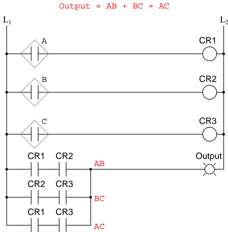
Either one of these circuits will adequately perform the task of operating the incinerator waste valve based on a flame verification from two out of the three flame sensors. At minimum, this is what we need to have a safe incinerator system. We can, however, extend the functionality of the system by adding to it logic circuitry designed to detect if any one of the sensors does not agree
