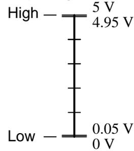
It should be obvious from these figures that CMOS gate circuits have far greater noise margins than TTL: 1.45 volts for CMOS low-level and high-level margins, versus a maximum of 0.7 volts for TTL. In other words, CMOS circuits can tolerate over twice the amount of superimposed "noise" voltage on their input lines before signal interpretation errors will result.
