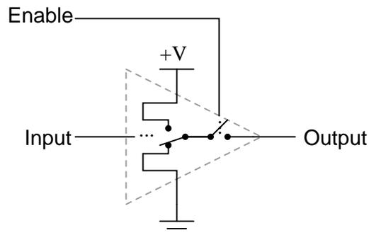
With the enable input held "high" (1), the buffer acts like an ordinary buffer with a totem pole output stage: it is capable of both sourcing and sinking current. However, the output terminal floats (goes into "high-Z" mode) if ever the enable input is grounded ("low"), regardless of the data signal's logic level. In other words, making the enable input terminal "low" (0) effectively *disconnects* the gate from whatever its output is wired to so that it can no longer have any effect.
