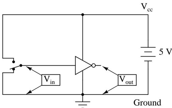
Power supply conductors are rarely shown in gate circuit schematics, even if the power supply connections at each gate are. Minimizing lines in our schematic, we get this:
