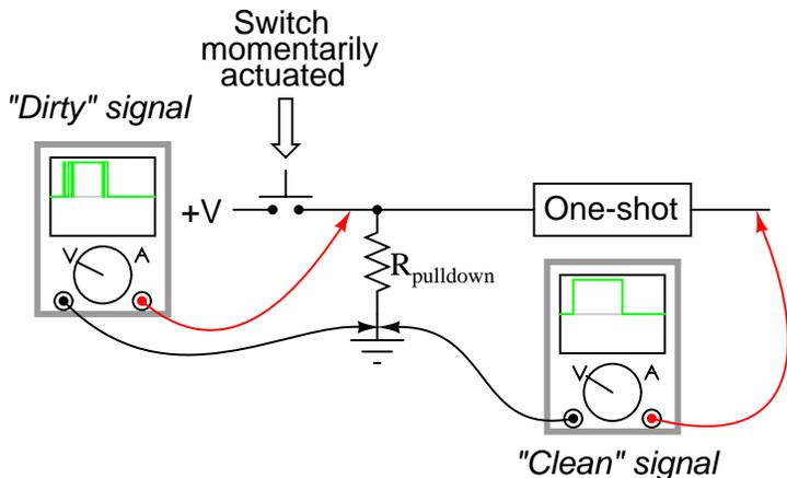
What if we only wanted a 10 second timed pulse output from a relay logic circuit, *regardless* of how many input pulses we received or how long-lived they may be? In that case, we'd have to couple a pulse-detector circuit to the retriggerable one-shot time delay circuit, like this:
