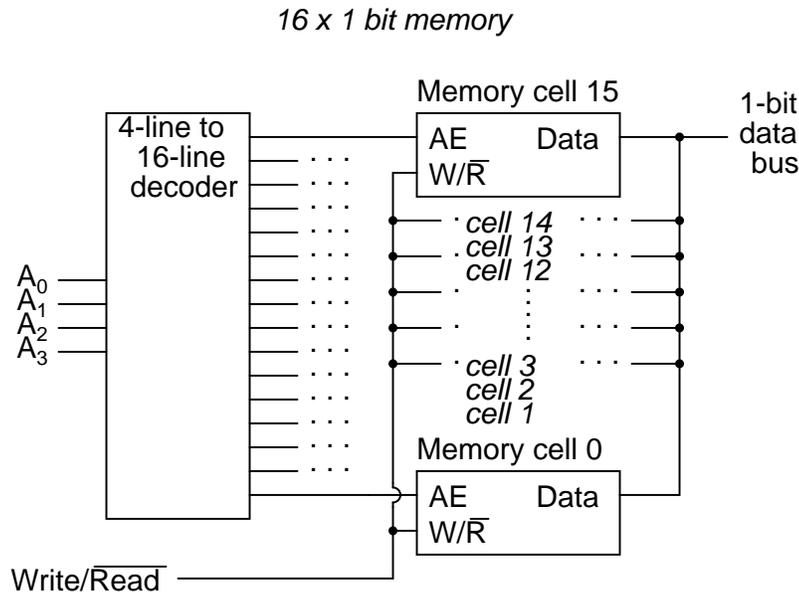
In the above circuit, 16 memory cells are individually addressed with a 4-bit binary code input into the decoder. If a cell is not addressed, it will be disconnected from the 1-bit data bus by its internal tristate buffers: consequently, data cannot be either written or read through the bus to or from that cell. Only the cell circuit that is addressed by the 4-bit decoder input will be accessible through the data bus.
