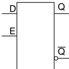
The D latch is nothing more than a gated S-R latch with an inverter added to make R the complement (inverse) of S. Let's explore the ladder logic equivalent of a D latch, modified from the basic ladder diagram of an S-R latch:
