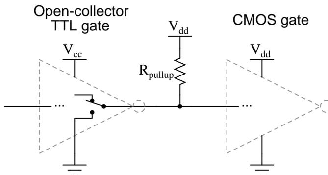
Although the CMOS gates used in the preceding examples were all inverters (single-input), the same principle of pullup and pulldown resistors applies to multiple-input CMOS gates. Of course, a separate pullup or pulldown resistor will be required for each gate input:
