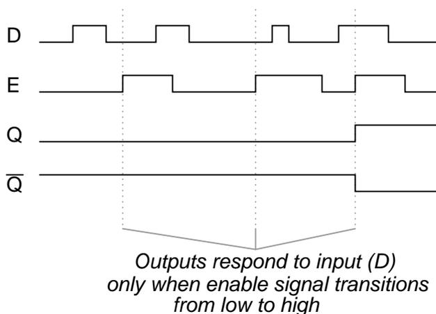
In the first timing diagram, the outputs respond to input D whenever the enable (E) input is high, for however long it remains high. When the enable signal falls back to a low state, the circuit remains latched. In the second timing diagram, we note a distinctly different response in the circuit output(s): it only responds to the D input during that brief moment of time when the enable signal *changes*, or *transitions*, from low to high. This is known as *positive* edge-triggering.
