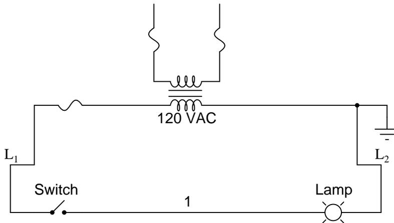
Here, the lamp (load) is located on the right-hand side of the rung, and so is the ground connection for the power source. This is no accident or coincidence; rather, it is a purposeful element of good design practice. Suppose that wire #1 were to accidentally come in contact with ground, the insulation of that wire having been rubbed off so that the bare conductor came in contact with grounded, metal conduit. Our circuit would now function like this:
