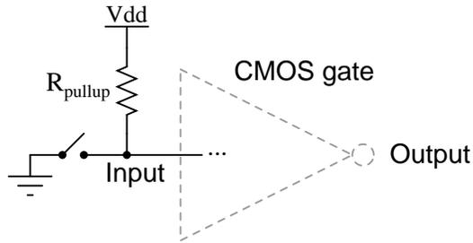
When switch is closed, the gate sees a definite "low" (0) input. When the switch is open,  $R_{pullup}$  will provide the connection to  $V_{dd}$  needed to secure a reliable "high" logic level for the CMOS gate input.
