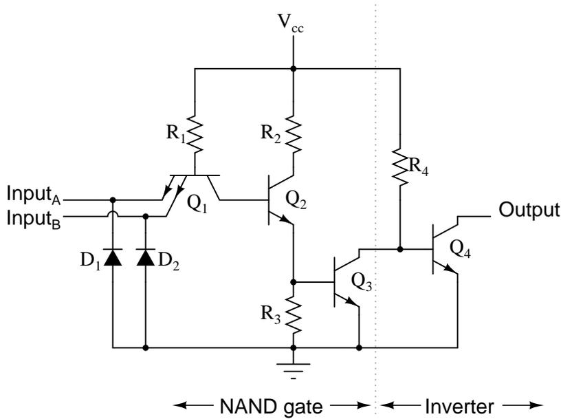
The truth table and equivalent gate circuit (an inverted-output NAND gate) are shown here:
