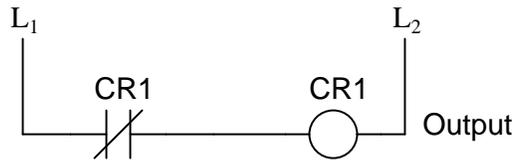
When the input is 0, the output switches to 1. That 1 output gets fed back to the input as a 1. When the input is 1, the output switches to 0. That 0 output gets fed back to the input as a 0, and the cycle repeats itself. The result is a high frequency (several megahertz) oscillator, if implemented with a solid-state (semiconductor) inverter gate:
