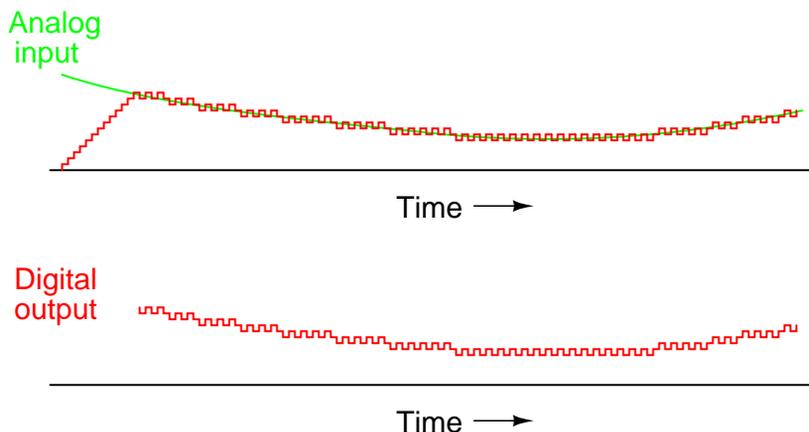
Note the much faster update time than any of the other "counting" ADC circuits. Also note how at the very beginning of the plot where the counter had to "catch up" with the analog signal, the rate of change for the output was identical to that of the first counting ADC. Also, with no shift register in this circuit, the binary output would actually ramp up rather than jump from zero to an accurate count as it did with the counter and successive approximation ADC circuits.
