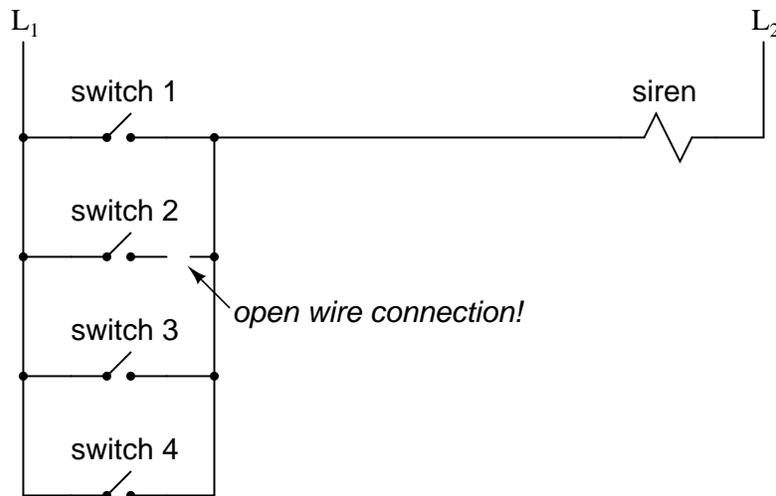
If this failure were to occur, the result would be that Switch #2 would no longer energize the siren if actuated. This, obviously, is not good in a fire alarm system. Unless the system were regularly tested (a good idea anyway), no one would know there was a problem until someone tried to use that switch in an emergency.
