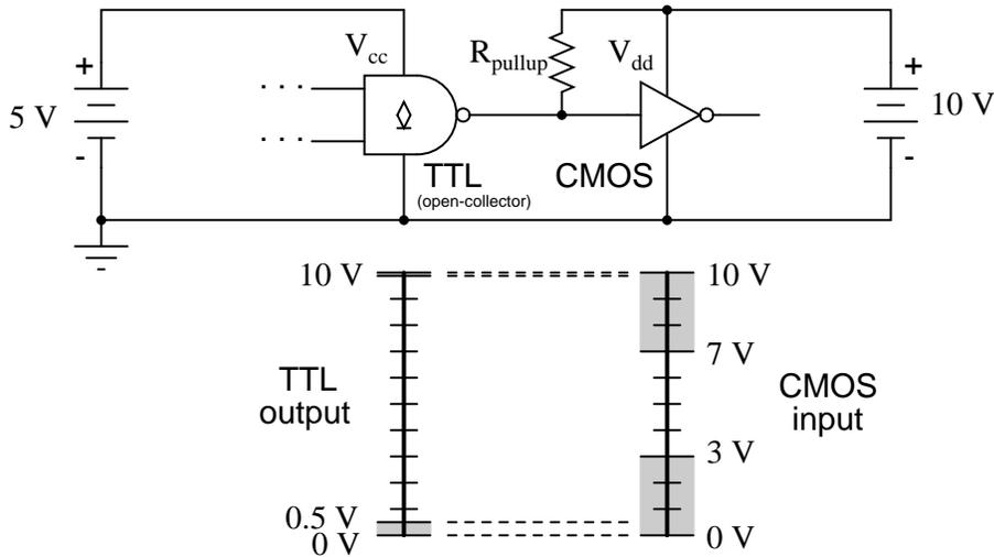
*Now, both "low" and "high" TTL signals are acceptable to the CMOS gate input*
