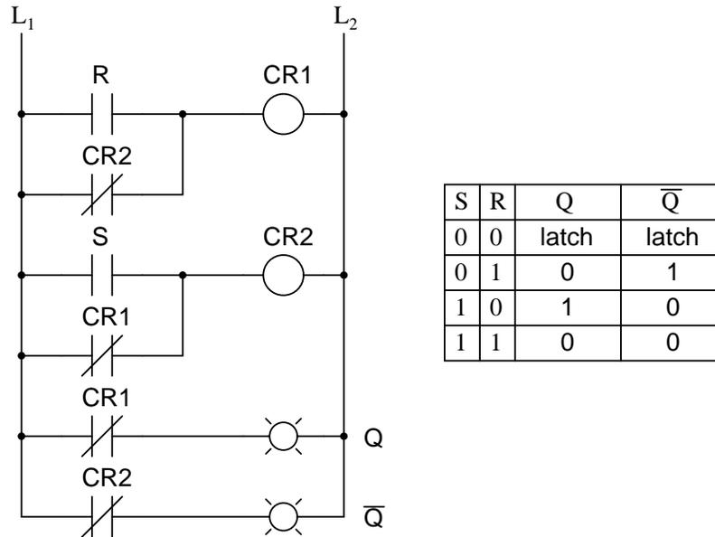
By definition, a condition of  $Q=1$  and  $\text{not-}Q=0$  is *set*. A condition of  $Q=0$  and  $\text{not-}Q=1$  is *reset*. These terms are universal in describing the output states of any multivibrator circuit.
