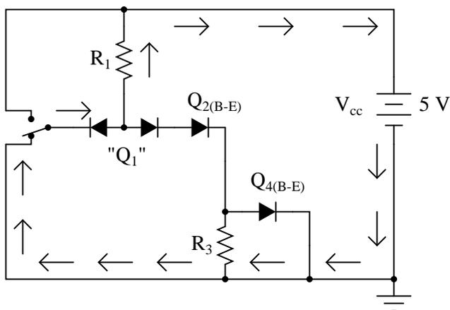
If we were to measure current in this circuit, we would find that *all* of the current goes through the left steering diode of  $Q_1$  and *none* of it through the right diode. Why is this? It still appears as though there is a complete path for current through  $Q_4$ 's diode,  $Q_2$ 's diode, the right diode of the pair, and  $R_1$ , so why will there be no current through that path?
