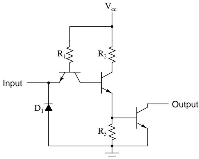
To designate open-collector output circuitry within a standard gate symbol, a special marker is used. Shown here is the symbol for an inverter gate with open-collector output:
