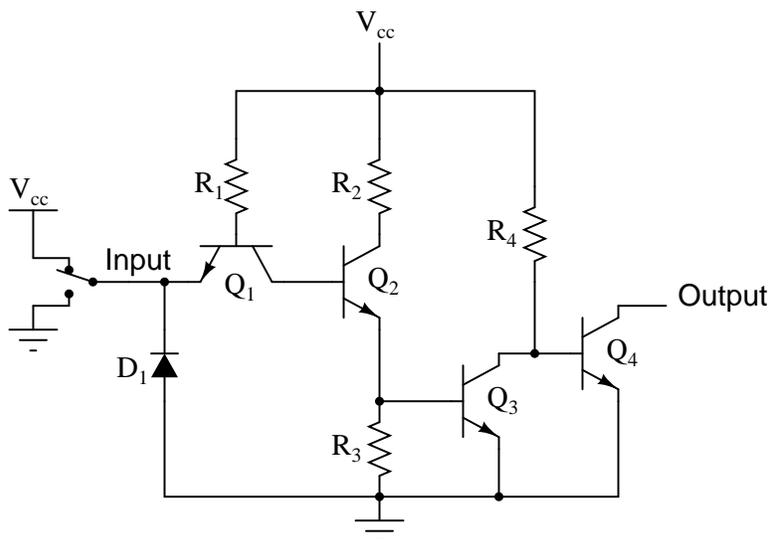
As before with the inverter circuit, the "high" input causes no conduction through the left steering diode of  $Q_1$  (emitter-to-base PN junction). All of  $R_1$ 's current goes through the base of transistor  $Q_2$ , saturating it:
