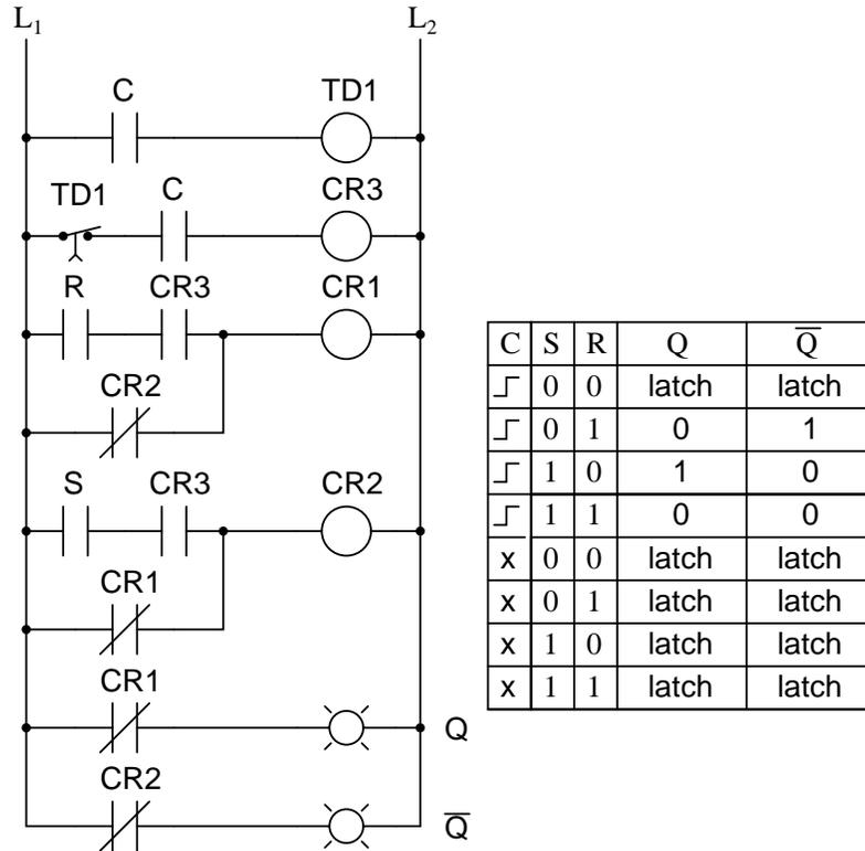
Relay contact CR<sub>3</sub> in the ladder diagram takes the place of the old E contact in the S-R latch circuit, and is closed only during the short time that both C is closed and time-delay contact TR<sub>1</sub> is closed. In either case (gate or ladder circuit), we see that the inputs S and R have no effect unless C is transitioning from a low (0) to a high (1) state. Otherwise, the flip-flop's outputs latch in their previous states.
