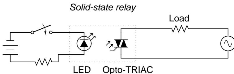
Being solid-state devices, there are no moving parts to wear out, and they are able to switch on and off much faster than any mechanical relay armature can move. There is no sparking between contacts, and no problems with contact corrosion. However, solid-state relays are still too expensive to build in very high current ratings, and so electromechanical contactors continue to dominate that application in industry today.
