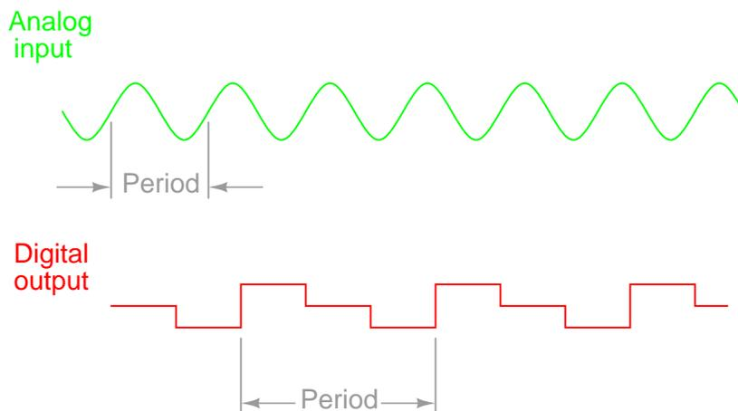
It should be understood that the Nyquist frequency is an *absolute* maximum frequency limit for an ADC, and does not represent the highest *practical* frequency measurable. To be safe, one shouldn't expect an ADC to successfully resolve any frequency greater than one-fifth to one-tenth
