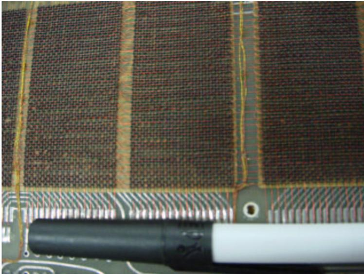
A core memory board of later design (circa 1971) is shown in the next photograph. Its cores are much smaller and more densely packed, giving more memory storage capacity than the former board (8 kbytes instead of 4 kbytes):
