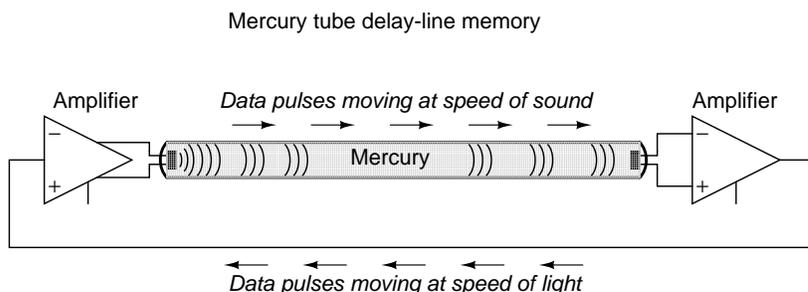
A feedback circuit connected to the receiving transducer would drive the transmitting transducer again, sending the same sequence of pulses through the tube as sound waves, storing the data as long as the feedback circuit continued to function. The delay line functioned like a first-in-first-out (FIFO) shift register, and external feedback turned that shift register behavior into a ring counter, cycling the bits around indefinitely.
