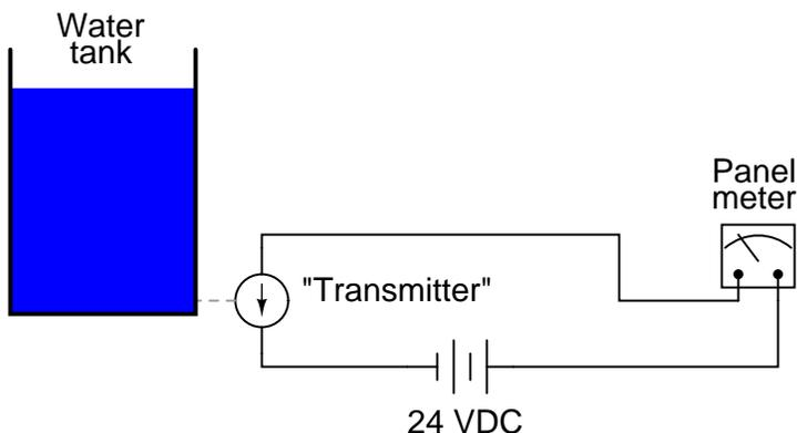
This analog communication system would be simple and robust. For many applications, it would suffice for our needs perfectly. But, it is not the *only* way to get the job done. For the purposes of exploring digital techniques, we'll explore other methods of monitoring this hypothetical tank, even though the analog method just described might be the most practical.
