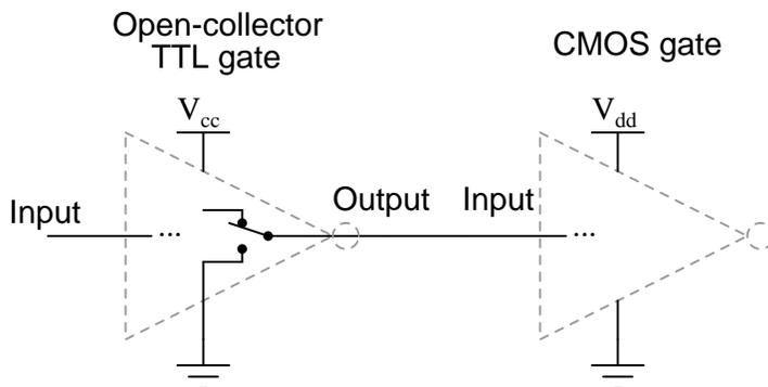
*When the open-collector TTL gate's output is "high" (1), the CMOS gate's input will be left floating and in an uncertain logic state.*
