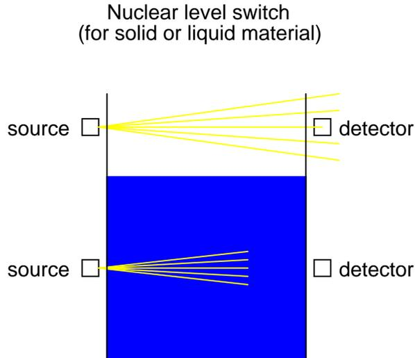
Both source and detector are outside of the vessel, with no intrusion at all except the radiation flux itself. The radioactive sources used are fairly weak and pose no immediate health threat to operations or maintenance personnel.
