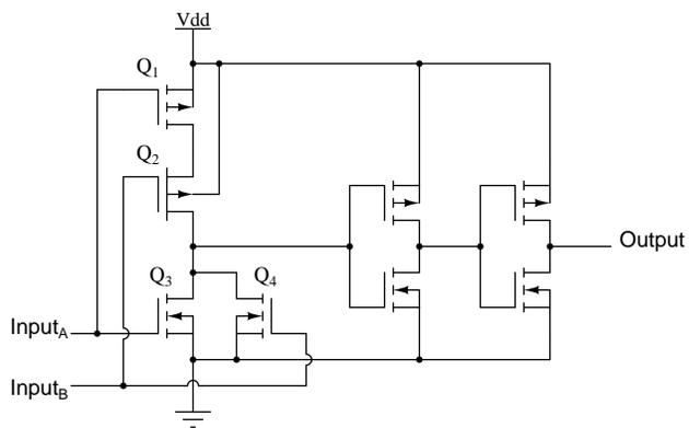
In essence, the B-series design enhancement adds two inverters to the output of a simple NOR circuit. This serves no purpose as far as digital logic is concerned, since two cascaded inverters simply cancel:
