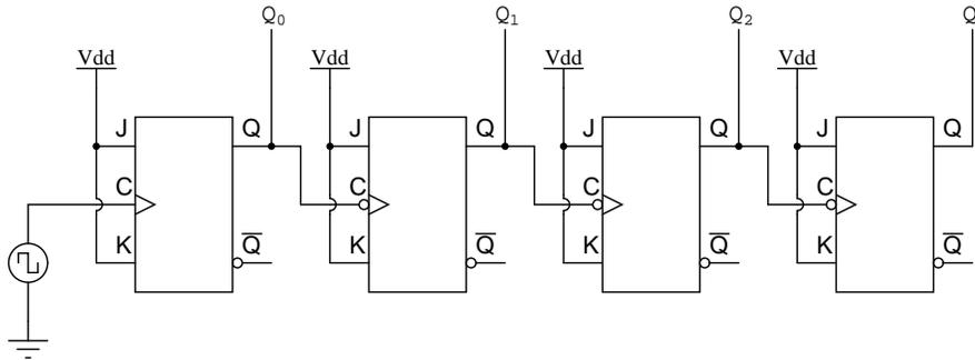
This circuit would yield the following output waveforms, when "clocked" by a repetitive source of pulses from an oscillator:
