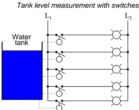
Each of these switches is wired to close a circuit, sending current to individual lamps mounted on a panel at the monitoring location. As each switch closed, its respective lamp would light, and whoever looked at the panel would see a 5-lamp representation of the tank's level.
