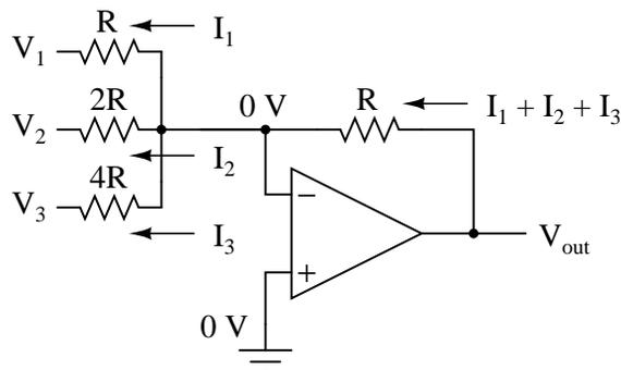
$$V_{\text{out}} = - \left( V_1 + \frac{V_2}{2} + \frac{V_3}{4} \right)$$
