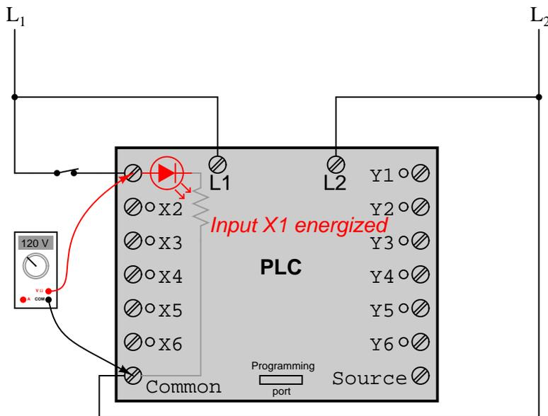
Output signals are generated by the PLC's computer circuitry activating a switching device (transistor, TRIAC, or even an electromechanical relay), connecting the "Source" terminal to any of the "Y-" labeled output terminals. The "Source" terminal, correspondingly, is usually connected to the L1 side of the 120 VAC power source. As with each input, an indicating LED on the front panel of the PLC gives visual indication of an "energized" output:
