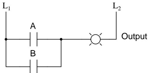
For each of the four possible combinations of input states (0-0, 0-1, 1-0, and 1-1), there is one, definite, unambiguous output state. Whether we're dealing with a multitude of cascaded gates or a single gate, that output state is determined by the truth table(s) for the gate(s) in the circuit, and nothing else.
