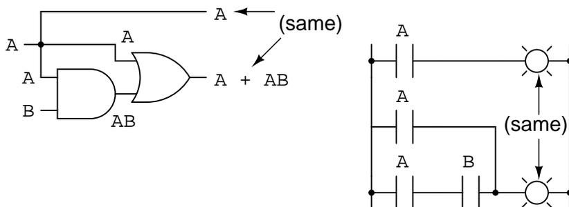
This rule may be proven symbolically by factoring an "A" out of the two terms, then applying the rules of  $A + 1 = 1$  and  $1A = A$  to achieve the final result:
