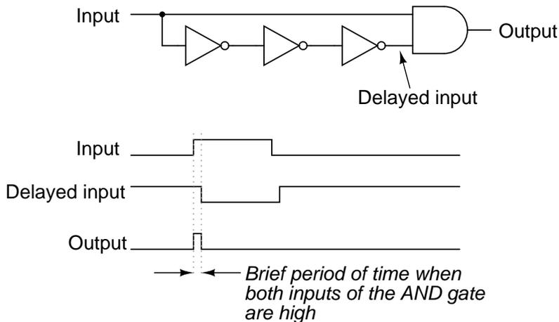
This circuit may be converted into a negative-edge pulse detector circuit with only a change of the final gate from AND to NOR:
