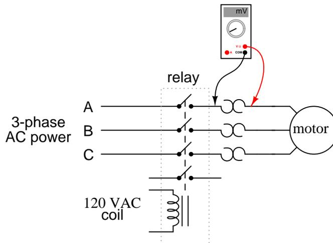
This is an especially useful trick to use for troubleshooting 3-phase AC motors, to see if one phase winding is burnt open or disconnected, which will result in a rapidly destructive condition known as "single-phasing." If one of the lines carrying power to the motor is open, it will not have any current through it (as indicated by a 0.00 mV reading across its heater), although the other two lines will (as indicated by small amounts of voltage dropped across the respective heaters).
