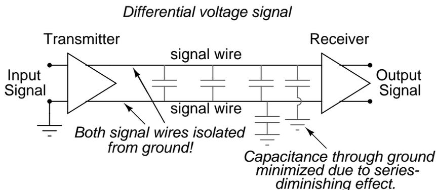
The triangular amplifier symbols represent *differential amplifiers*, which output a voltage signal between two wires, neither one electrically common with ground. Having eliminated any relation between the voltage signal and ground, the only significant capacitance imposed on the signal voltage is that existing between the two signal wires. Capacitance between a signal wire and a grounded conductor is of much less effect, because the capacitive path between the two signal wires via a
