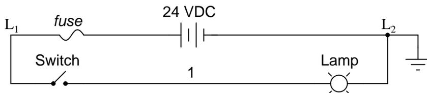
So long as the switch contacts and relay coils are all adequately rated, it really doesn't matter what level of voltage is chosen for the system to operate with.
