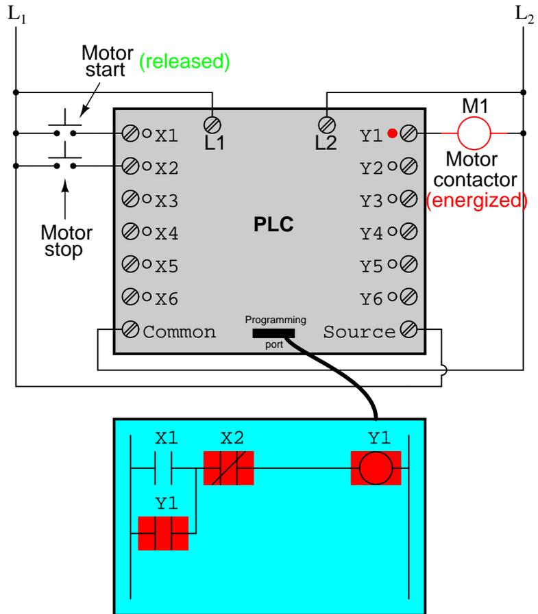
To stop the motor, we must momentarily press the "Stop" pushbutton, which will energize the X2 input and "open" the normally-closed "contact," breaking continuity to the Y1 "coil:"
