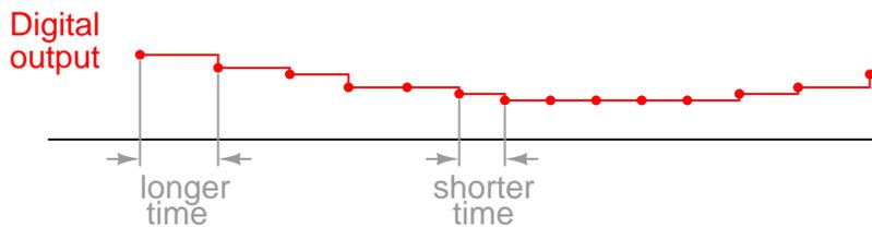
For many ADC applications, this variation in update frequency (sample time) would not be acceptable. This, and the fact that the circuit's need to count all the way from 0 at the beginning of each count cycle makes for relatively slow sampling of the analog signal, places the digital-ramp ADC at a disadvantage to other counter strategies.
