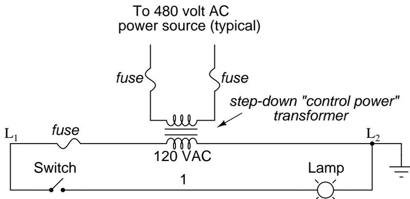
Typically in industrial relay logic circuits, but not always, the operating voltage for the switch contacts and relay coils will be 120 volts AC. Lower voltage AC and even DC systems are sometimes built and documented according to "ladder" diagrams:
