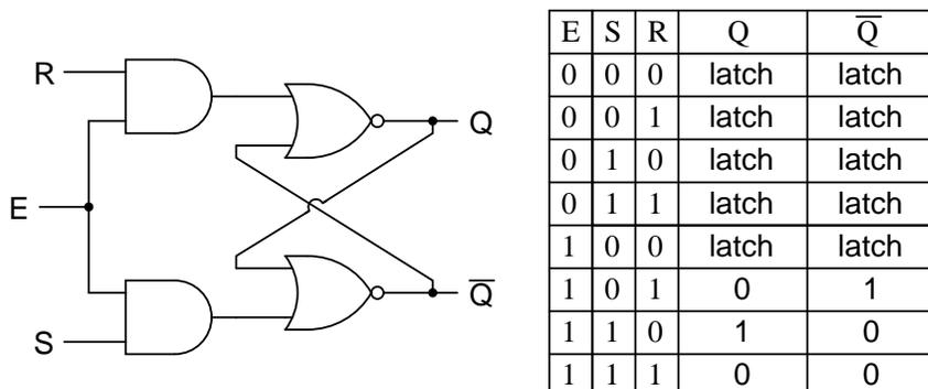
When the  $E=0$ , the outputs of the two AND gates are forced to 0, regardless of the states of either S or R. Consequently, the circuit behaves as though S and R were both 0, latching the Q and not-Q outputs in their last states. Only when the enable input is activated (1) will the latch respond to the S and R inputs. Note the identical function in ladder logic:
