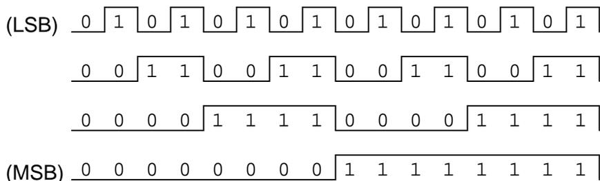
J-K flip-flops are ideally suited for this task, because they have the ability to "toggle" their output state at the command of a clock pulse when both J and K inputs are made "high" (1):
