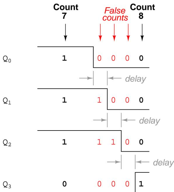
Instead of cleanly transitioning from a "0111" output to a "1000" output, the counter circuit will very quickly ripple from 0111 to 0110 to 0100 to 0000 to 1000, or from 7 to 6 to 4 to 0 and then to 8. This behavior earns the counter circuit the name of *ripple counter*, or *asynchronous counter*.
