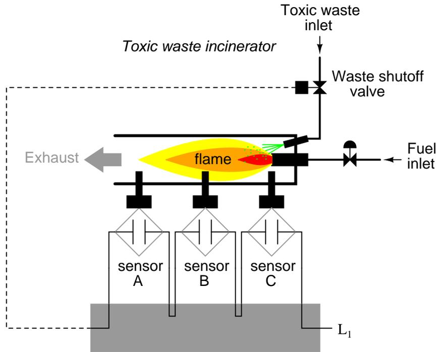
While this design strategy maximizes safety, it makes the system very susceptible to sensor failures of the opposite kind. Suppose that one of the three sensors were to fail in such a way that it indicated no flame when there really was a good flame in the incinerator's combustion chamber. That single failure would shut off the waste valve unnecessarily, resulting in lost production time and wasted fuel (feeding a fire that wasn't being used to incinerate waste).
