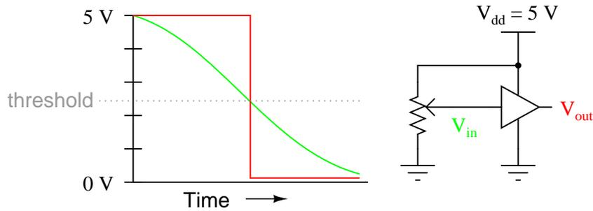
In the presence of AC "noise" voltage superimposed on the DC input signal, a single threshold point at which the gate alters its interpretation of logic level will result in an erratic output:
