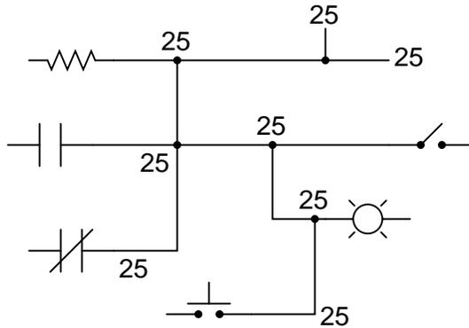
In ladder diagrams, the load device (lamp, relay coil, solenoid coil, etc.) is almost always drawn at the right-hand side of the rung. While it doesn't matter electrically where the relay coil is located within the rung, it *does* matter which end of the ladder's power supply is grounded, for reliable operation.
