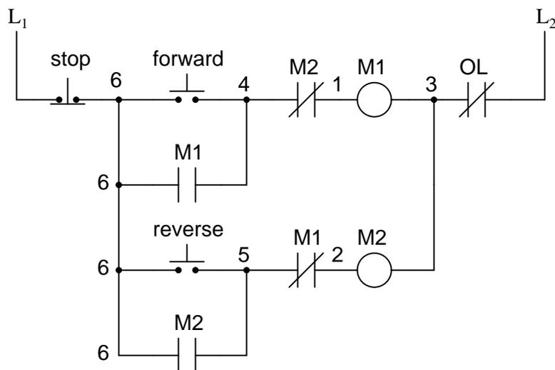
Now, if either forward or reverse circuits are latched, they may be "unlatched" by momentarily pressing the "Stop" pushbutton, which will open either forward or reverse circuit, de-energizing the energized contactor, and returning the seal-in contact to its normal (open) state. The "Stop" switch, having normally-closed contacts, will conduct power to either forward or reverse circuits when released.
