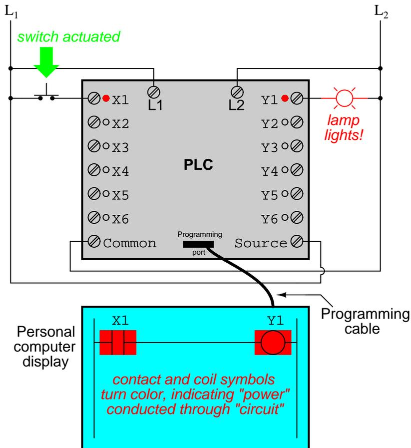
It must be understood that the X1 contact, Y1 coil, connecting wires, and "power" appearing in the personal computer's display are all *virtual*. They do not exist as real electrical components. They exist as commands in a computer program – a piece of software only – that just happens to resemble a real relay schematic diagram.
