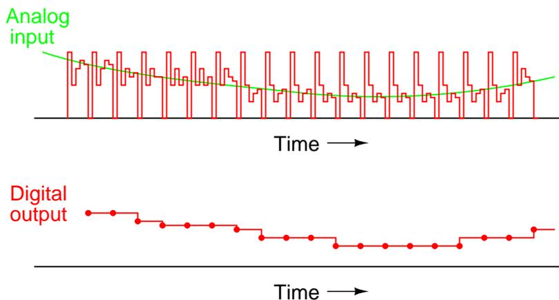
Note how the updates for this ADC occur at regular intervals, unlike the digital ramp ADC circuit.
