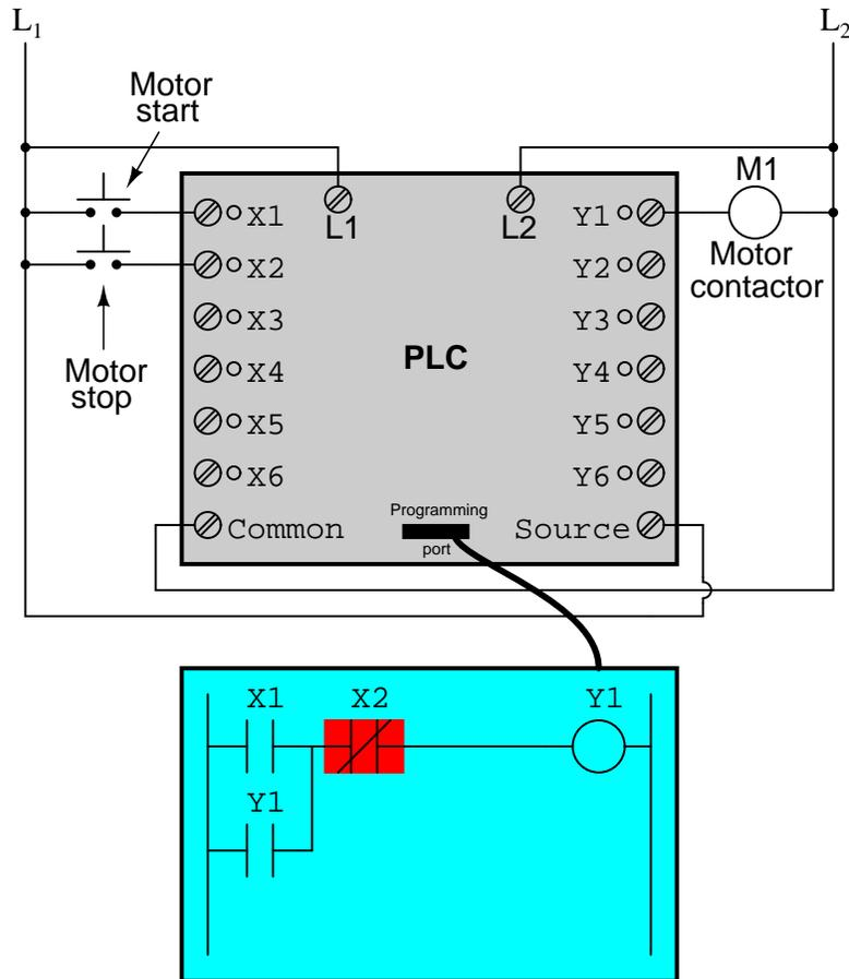
The pushbutton switch connected to input X1 serves as the "Start" switch, while the switch connected to input X2 serves as the "Stop." Another contact in the program, named Y1, uses the output coil status as a seal-in contact, directly, so that the motor contactor will continue to be energized after the "Start" pushbutton switch is released. You can see the normally-closed contact X2 appear in a colored block, showing that it is in a closed ("electrically conducting") state.
