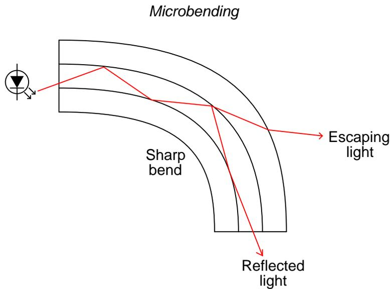
Not only does microbending lead to diminished signal strength due to the lost light, but it also constitutes a security weakness in that a light sensor intentionally placed on the outside of a sharp bend could intercept digital data transmitted over the fiber.
