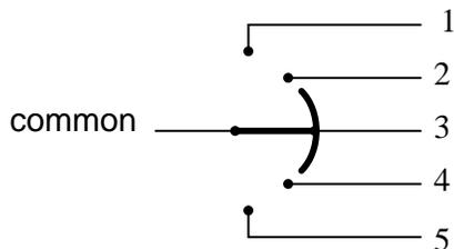
When movable contact(s) can be brought into one of several positions with stationary contacts, those positions are sometimes called *throws*. The number of movable contacts is sometimes called *poles*. Both selector switches shown above with one moving contact and five stationary contacts would be designated as "single-pole, five-throw" switches.
