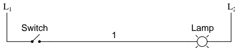
The " $L_1$ " and " $L_2$ " designations refer to the two poles of a 120 VAC supply, unless otherwise noted.  $L_1$  is the "hot" conductor, and  $L_2$  is the grounded ("neutral") conductor. These designations have nothing to do with inductors, just to make things confusing. The actual transformer or generator supplying power to this circuit is omitted for simplicity. In reality, the circuit looks something like this:
