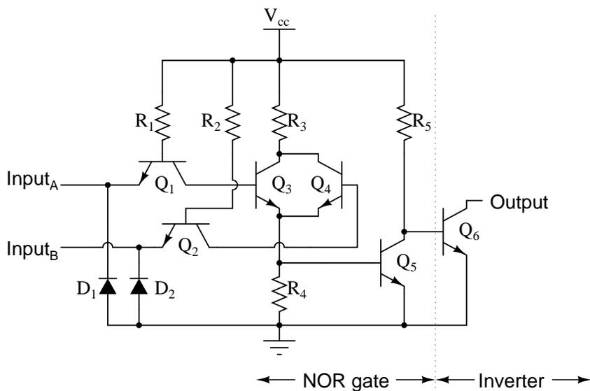
The truth table and equivalent gate circuit (an inverted-output NOR gate) are shown here:
