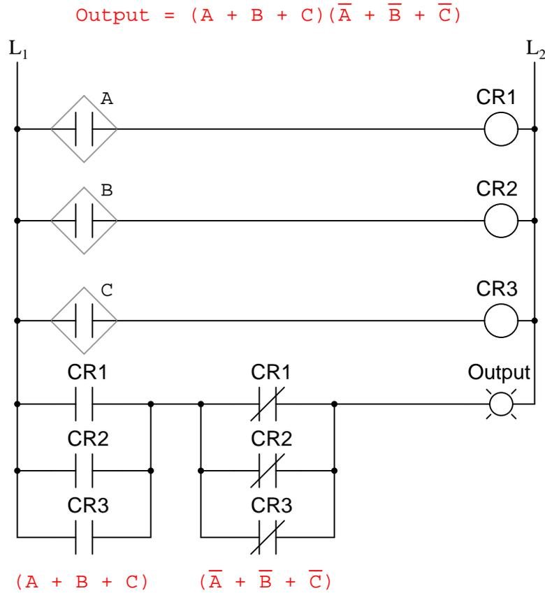
The previous two circuits represent different versions of the "sensor disagreement" logic circuit only, not the "good flame" detection circuit(s). The entire logic system would be the combination of both "good flame" and "sensor disagreement" circuits, shown on the same diagram.
