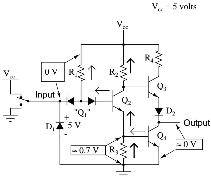
With  $Q_4$  saturated, the output terminal will be almost directly shorted to ground, leaving the output terminal at a voltage (in reference to ground) of almost 0 volts, or a binary "0" ("low") logic
