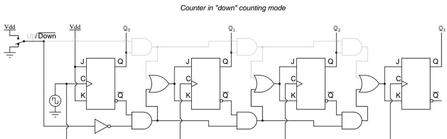
Up/down counter circuits are very useful devices. A common application is in machine motion control, where devices called *rotary shaft encoders* convert mechanical rotation into a series of electrical pulses, these pulses "clocking" a counter circuit to track total motion:
