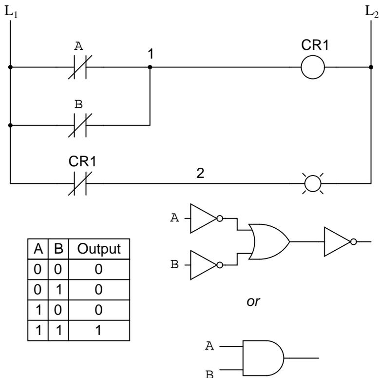
From the switches to the coil of  $CR_1$ , the logical function is that of a NAND gate.  $CR_1$ 's normally-closed contact provides one final inversion to turn the NAND function into an AND function.
