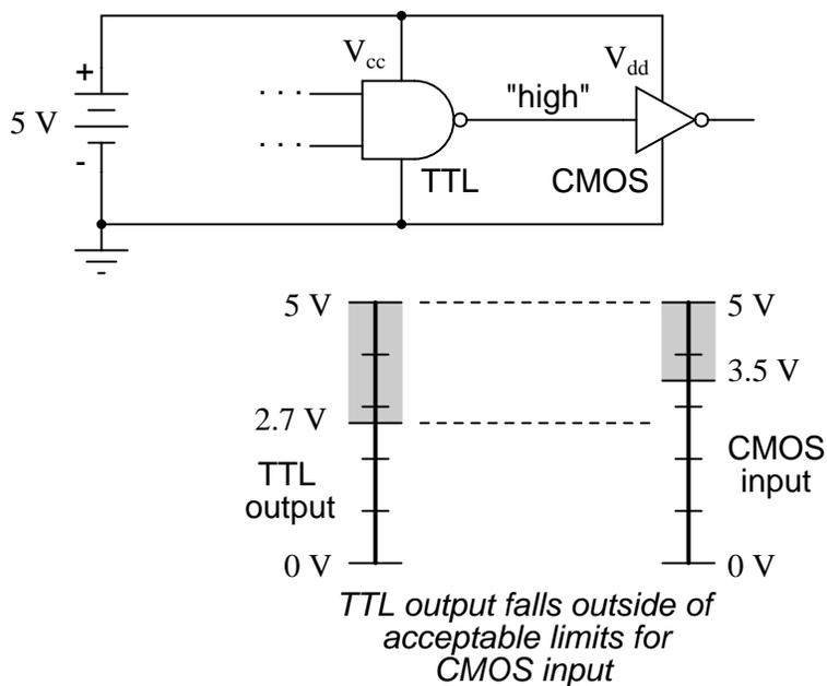
Given this mismatch, it is entirely possible for the TTL gate to output a valid "high" signal (valid, that is, according to the standards for TTL) that lies within the "uncertain" range for the CMOS input, and may be (falsely) interpreted as a "low" by the receiving gate. An easy "fix" for this problem is to augment the TTL gate's "high" signal voltage level by means of a pullup resistor:
