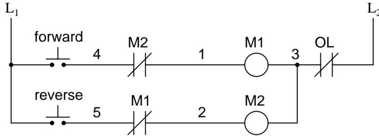
Now, when  $M_1$  is energized, the normally-closed auxiliary contact on the second rung will be open, thus preventing  $M_2$  from being energized, even if the "Reverse" pushbutton is actuated. Likewise,  $M_1$ 's energization is prevented when  $M_2$  is energized. Note, as well, how additional wire numbers (4 and 5) were added to reflect the wiring changes.
