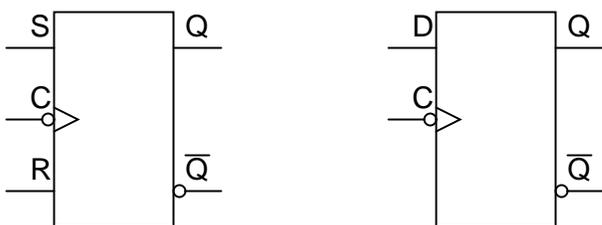
Both of the above flip-flops will "clock" on the falling edge (high-to-low transition) of the clock signal.
