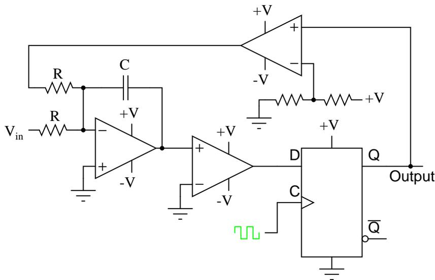
The leftmost op-amp is the (summing) integrator. The next op-amp the integrator feeds into is the comparator, or 1-bit ADC. Next comes the D-type flip-flop, which latches the comparator's output at every clock pulse, sending either a "high" or "low" signal to the next comparator at the top of the circuit. This final comparator is necessary to convert the single-polarity 0V / 5V logic level output voltage of the flip-flop into a +V / -V voltage signal to be fed back to the integrator.
