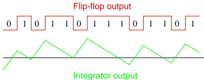
A parallel binary number output is obtained from this circuit by averaging the serial stream of bits together. For example, a counter circuit could be designed to collect the total number of 1's output by the flip-flop in a given number of clock pulses. This count would then be indicative of the analog input voltage.
