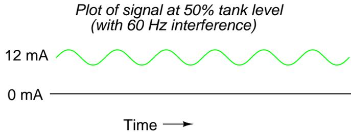
The above example is a bit exaggerated, but the concept should be clear: *any* electrical noise introduced into an analog measurement system will be interpreted as changes in the measured quantity. One way to combat this problem is to symbolize the tank's water level by means of a digital signal instead of an analog signal. We can do this really crudely by replacing the analog transmitter device with a set of water level switches mounted at different heights on the tank:
