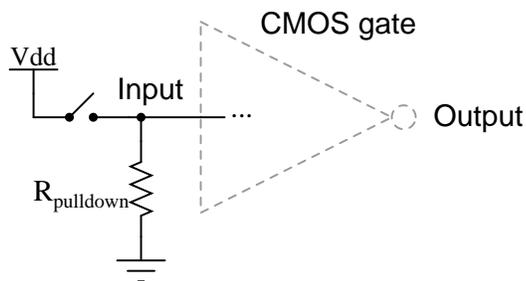
When switch is closed, the gate sees a definite "high" (1) input. When the switch is open,  $R_{pulldown}$  will provide the connection to ground needed to secure a reliable "low" logic level for the CMOS gate input.
