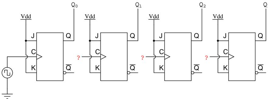
If we used flip-flops with negative-edge triggering (bubble symbols on the clock inputs), we could simply connect the clock input of each flip-flop to the Q output of the flip-flop before it, so that when the bit before it changes from a 1 to a 0, the "falling edge" of that signal would "clock" the next flip-flop to toggle the next bit:
