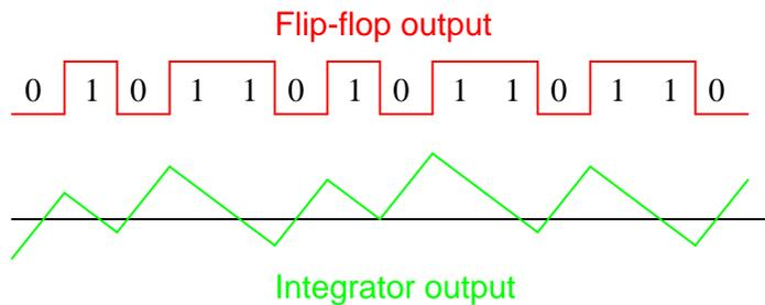
As the analog input signal increases in magnitude, so does the occurrence of 1's in the digital output of the flip-flop:
