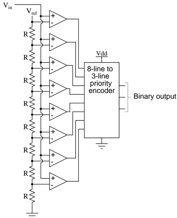
$V_{ref}$  is a stable reference voltage provided by a precision voltage regulator as part of the converter circuit, not shown in the schematic. As the analog input voltage exceeds the reference voltage at each comparator, the comparator outputs will sequentially saturate to a high state. The priority encoder generates a binary number based on the highest-order active input, ignoring all other active inputs.
