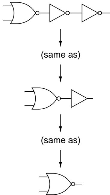
However, adding these inverter stages to the circuit does serve the purpose of increasing overall voltage gain, making the output more sensitive to changes in input state, working to overcome the inherent slowness caused by CMOS gate input capacitance.
