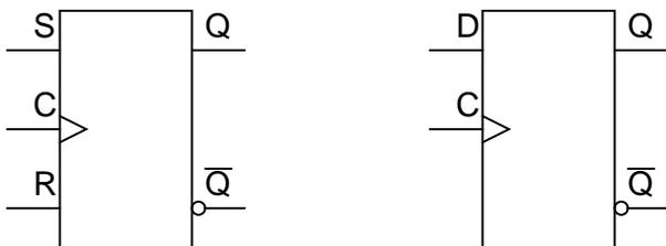
The triangle symbol next to the clock inputs tells us that these are edge-triggered devices, and consequently that these are flip-flops rather than latches. The symbols above are positive edge-triggered: that is, they "clock" on the rising edge (low-to-high transition) of the clock signal. Negative edge-triggered devices are symbolized with a bubble on the clock input line:
