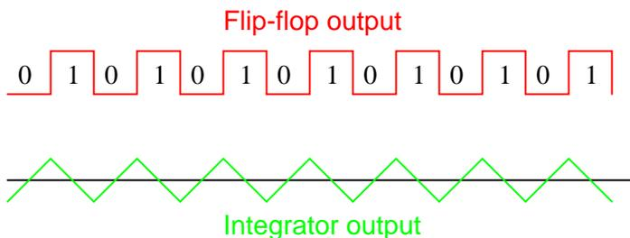
If, however, we apply a negative analog input voltage, the integrator will have a tendency to ramp its output in a positive direction. Feedback can only add to the integrator's ramping by a fixed voltage over a fixed time, and so the bit stream output by the flip-flop will not be quite the same:
