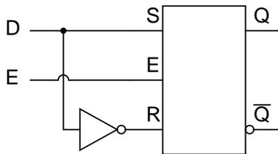
Like both the S-R and gated S-R latches, the D latch circuit may be found as its own prepackaged circuit, complete with a standard symbol:
