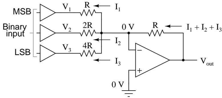
If we chart the output voltages for all eight combinations of binary bits (000 through 111) input to this circuit, we will get the following progression of voltages:
