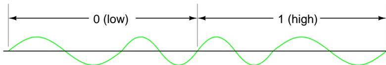
With sine wave signal voltages, many of the problems encountered with square wave digital signals are minimized, although the circuitry required to modulate (and demodulate) the network signals is more complex and expensive.
