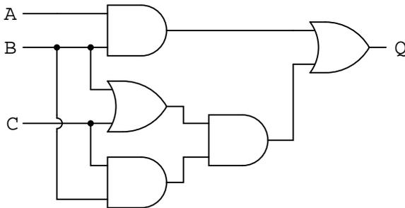
Our first step in simplification must be to write a Boolean expression for this circuit. This task is easily performed step by step if we start by writing sub-expressions at the output of each gate, corresponding to the respective input signals for each gate. Remember that OR gates are equivalent to Boolean addition, while AND gates are equivalent to Boolean multiplication. For example, I'll write sub-expressions at the outputs of the first three gates:
