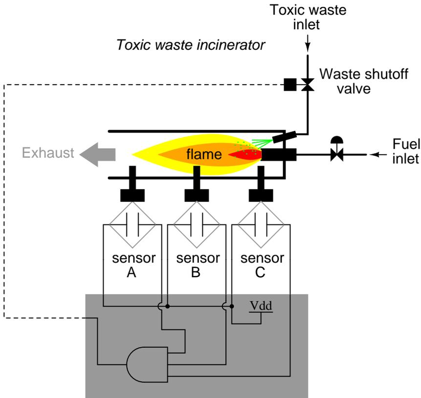
If using relay circuitry, we could create this AND function by wiring three relay contacts in series, or simply by wiring the three sensor contacts in series, so that the only way electrical power could be sent to open the waste valve is if all three sensors indicate flame:
