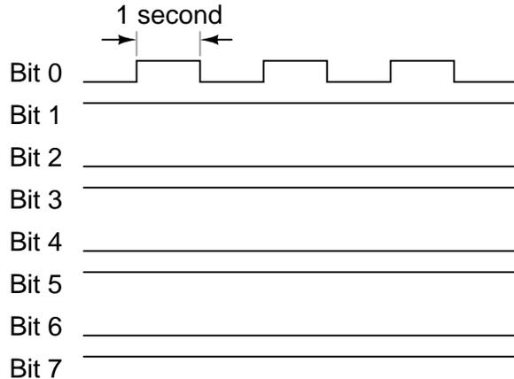
Since only the least significant bit (Bit 1) is changing, the frequency on that wire (to ground) is only 1/2 Hertz. In fact, no matter what numbers are being generated by the A/D converter between updates, the frequency on any wire in this modified BogusBus network cannot exceed 1/2 Hertz, because that's how fast the A/D updates its digital output. 1/2 Hertz is pretty slow, and should present no problems for our network wiring.
