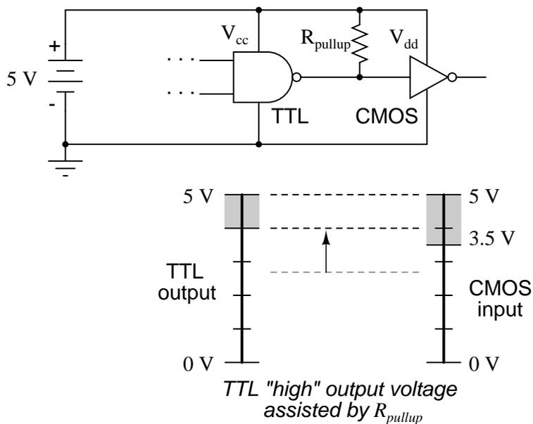
Something more than this, though, is required to interface a TTL output with a CMOS input, if the receiving CMOS gate is powered by a greater power supply voltage:
