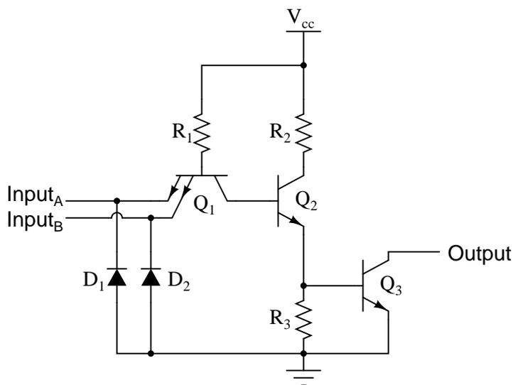
In the single-input (inverter) circuit, grounding the input resulted in an output that assumed the "high" (1) state. In the case of the open-collector output configuration, this "high" state was simply "floating." Allowing the input to float (or be connected to  $V_{cc}$ ) resulted in the output becoming grounded, which is the "low" or 0 state. Thus, a 1 in resulted in a 0 out, and visa-versa.
