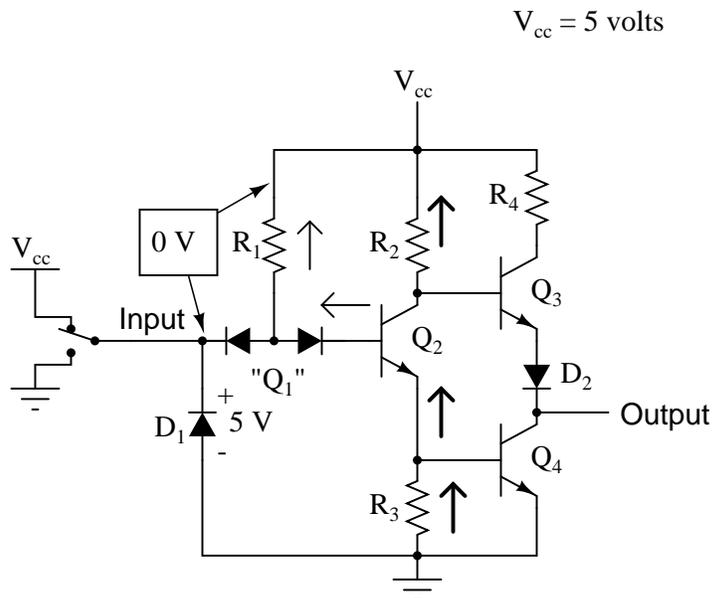
With base current provided, transistor  $Q_2$  will be turned "on." More specifically, it will be *saturated* by virtue of the more-than-adequate current allowed by  $R_1$  through the base. With  $Q_2$  saturated, resistor  $R_3$  will be dropping enough voltage to forward-bias the base-emitter junction of transistor  $Q_4$ , thus saturating it as well:
