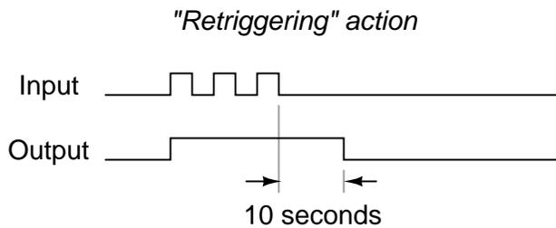
One application for a retriggerable one-shot is that of a single mechanical contact debouncer. As you can see from the above timing diagram, the output will remain high despite "bouncing" of the input signal from a mechanical switch. Of course, in a real-life switch debouncer circuit, you'd probably want to use a time delay of much shorter duration than 10 seconds, as you only need to "debounce" pulses that are in the millisecond range.
