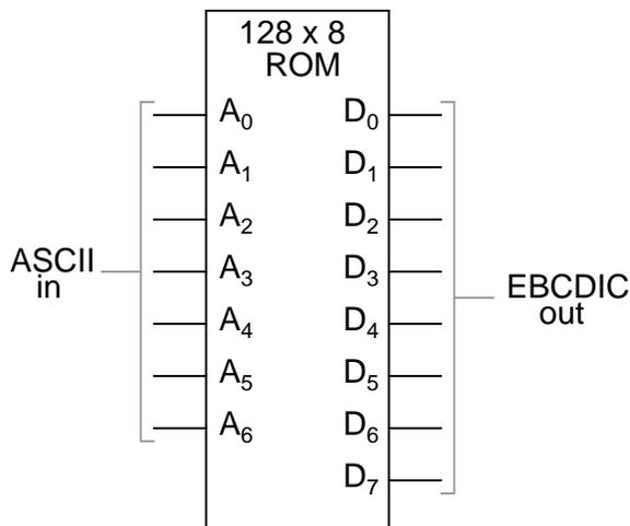
Again, all that is required is for the ROM chip to be properly programmed with the necessary data so that each valid ASCII input will produce a corresponding EBCDIC output code.
