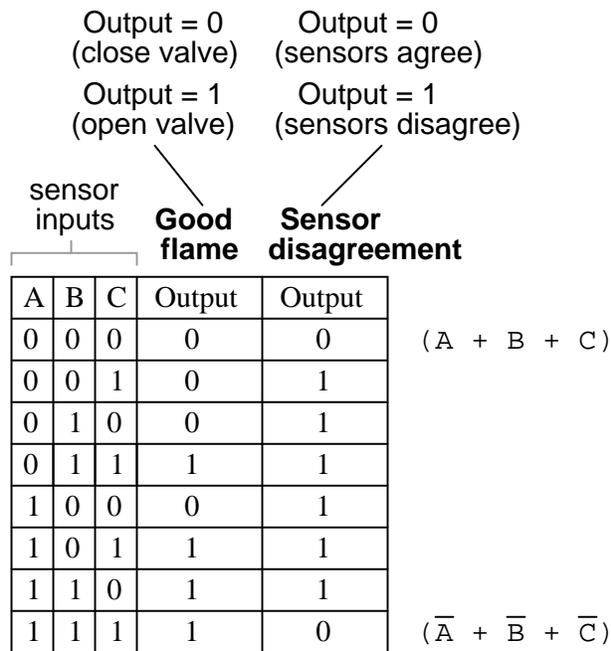
$Output = (A + B + C)(\bar{A} + \bar{B} + \bar{C})$
