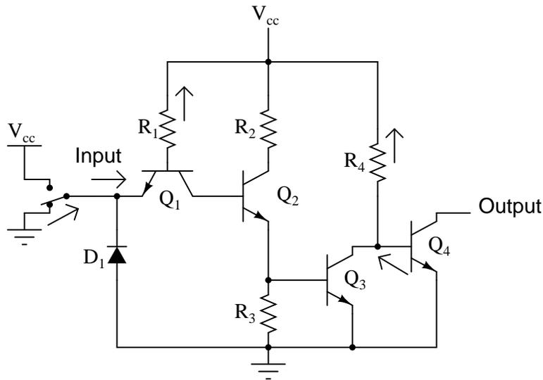
All of  $R_1$ 's current is now diverted through the input switch, thus eliminating base current through  $Q_2$ . This forces transistor  $Q_2$  into cutoff so that no base current goes through  $Q_3$  either. With  $Q_3$  cutoff as well,  $Q_4$  is will be saturated by the current through resistor  $R_4$ , thus connecting the output terminal to ground, making it a "low" logic level. Thus, a "low" input gives a "low"
