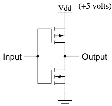
Notice the " $V_{dd}$ " label on the positive power supply terminal. This label follows the same convention as " $V_{cc}$ " in TTL circuits: it stands for the constant voltage applied to the drain of a field effect transistor, in reference to ground.
