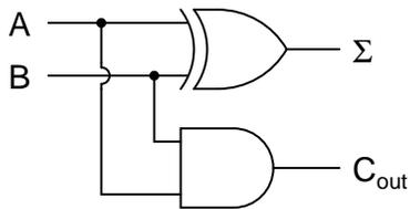
The  $\Sigma$  symbol represents the "sum" output of the half-adder, the sum's least significant bit (LSB).  $C_{out}$  represents the "carry" output of the half-adder, the sum's most significant bit (MSB).
