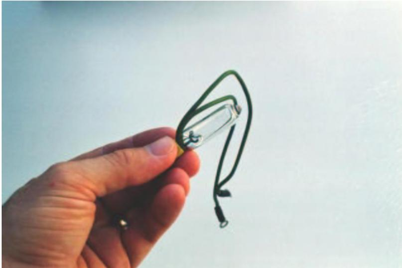
Mercury switch contacts are impractical to build in large sizes, and so you will typically find such contacts rated at no more than a few amps, and no more than 120 volts. There are exceptions, of course, but these are common limits.
