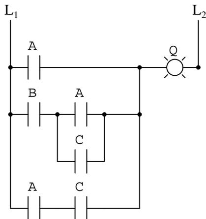
As before, our first step in reducing this circuit to its simplest form must be to develop a Boolean expression from the schematic. The easiest way I've found to do this is to follow the same steps I'd normally follow to reduce a series-parallel resistor network to a single, total resistance. For example, examine the following resistor network with its resistors arranged in the same connection pattern as the relay contacts in the former circuit, and corresponding total resistance formula:
