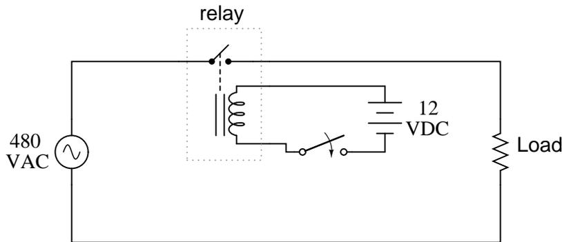
In the above schematic, the relay's coil is energized by the low-voltage (12 VDC) source, while the single-pole, single-throw (SPST) contact interrupts the high-voltage (480 VAC) circuit. It is quite likely that the current required to energize the relay coil will be hundreds of times less than the current rating of the contact. Typical relay coil currents are well below 1 amp, while typical contact ratings for industrial relays are at least 10 amps.
