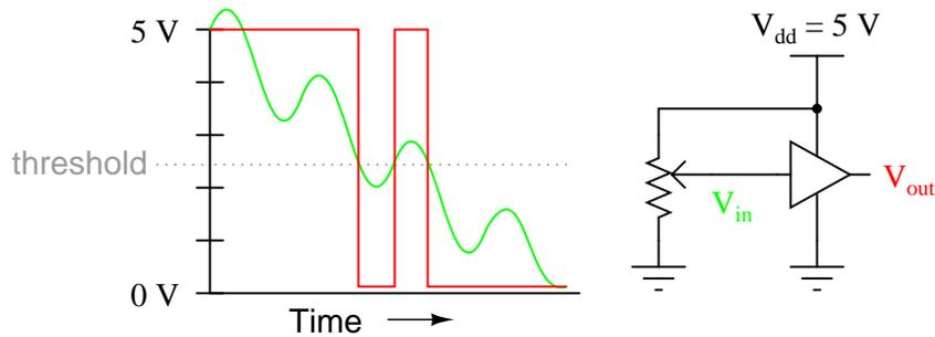
If this scenario looks familiar to you, it's because you remember a similar problem with (analog) voltage comparator op-amp circuits. With a single threshold point at which an input causes the output to switch between "high" and "low" states, the presence of significant noise will cause erratic changes in the output:
