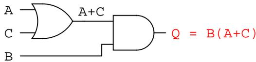
Obviously, this circuit is much simpler than the original, having only two logic gates instead of five. Such component reduction results in higher operating speed (less delay time from input signal transition to output signal transition), less power consumption, less cost, and greater reliability.
