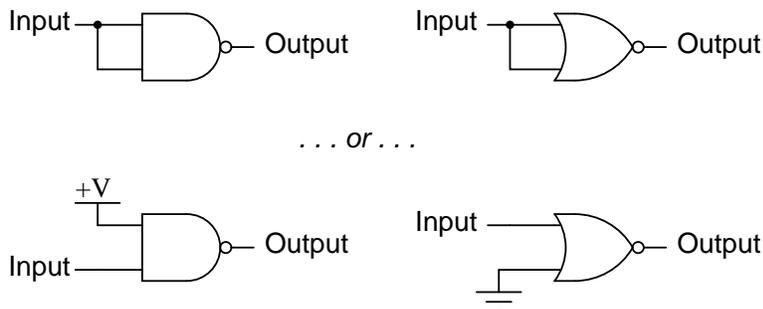
As you can see, there are two ways to use a NAND gate as an inverter, and two ways to use a NOR gate as an inverter. Either method works, although connecting TTL inputs together increases the amount of current loading to the driving gate. For CMOS gates, common input terminals decreases the switching speed of the gate due to increased input capacitance.
