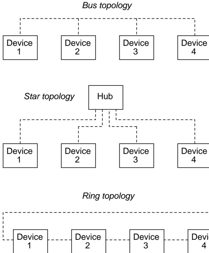
Many network standards dictate the type of topology which is used, while others are more versatile. Ethernet, for example, is commonly implemented in a "bus" topology but can also be implemented in a "star" or "ring" topology with the appropriate interconnecting equipment. Other networks, such as RS-232C, are almost exclusively point-to-point; and token ring (as you might have guessed) is implemented solely in a ring topology.
