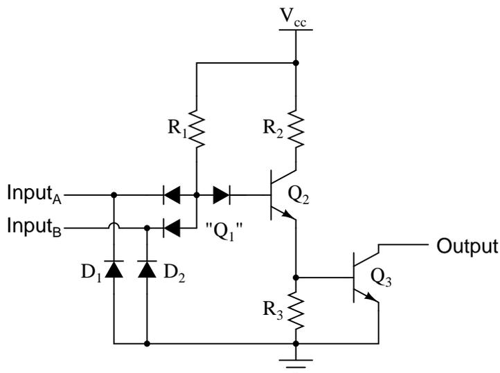
This schematic illustrates a real circuit, but it isn't called a "two-input inverter." Through analysis we will discover what this circuit's logic function is and correspondingly what it should be designated as.
