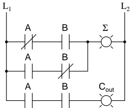
Either circuit is capable of adding two binary digits together. The mathematical "rules" of
