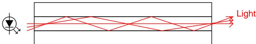
A light pulse emitted by the LED taking a shorter path through the fiber will arrive at the detector sooner than light pulses taking longer paths. The result is distortion of the square-wave's rising and falling edges, called *pulse stretching*. This problem becomes worse as the overall fiber length is increased:
