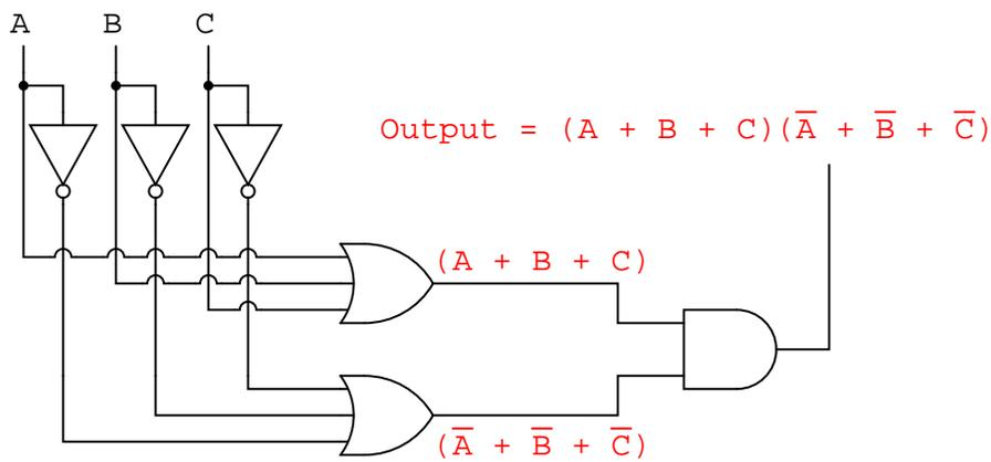
Correspondingly, whereas a Sum-Of-Products expression could be implemented as a parallel collection of series-connected relay contacts, a Product-Of-Sums expression can be implemented as a series collection of parallel-connected relay contacts:
