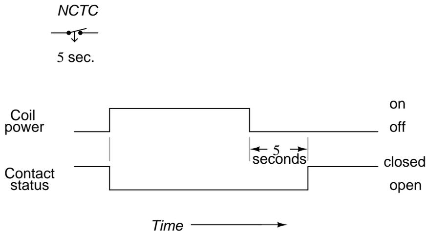
Time-delay relays are very important for use in industrial control logic circuits. Some examples of their use include:
