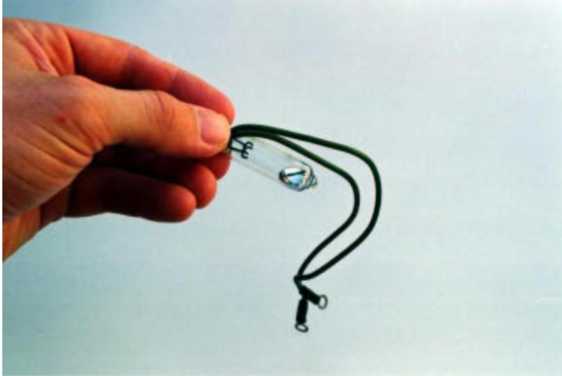
Here, the same switch is shown in the closed position. Gravity now holds the liquid mercury in contact with the two metal contacts, providing electrical continuity from one to the other:
