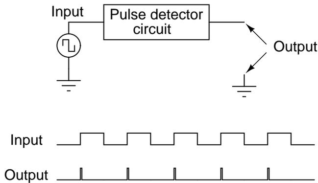
The duration of each output pulse is set by components in the pulse circuit itself. In ladder logic, this can be accomplished quite easily through the use of a time-delay relay with a very short delay time:
