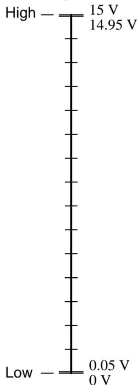
The margins for acceptable "high" and "low" signals may be greater than what is shown in the previous illustrations. What is shown represents "worst-case" input signal performance, based on manufacturer's specifications. In practice, it may be found that a gate circuit will tolerate "high" signals of considerably less voltage and "low" signals of considerably greater voltage than those specified here.
