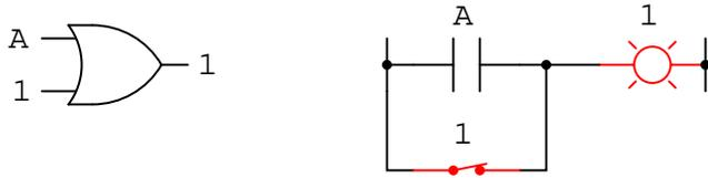
No matter what the value of  $A$ , the sum of  $A$  and  $1$  will always be  $1$ . In a sense, the "1" signal *overrides* the effect of  $A$  on the logic circuit, leaving the output fixed at a logic level of  $1$ .
