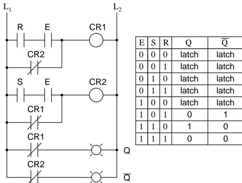
A practical application of this might be the same motor control circuit (with two normally-open pushbutton switches for *start* and *stop*), except with the addition of a master lockout input (E) that disables both pushbuttons from having control over the motor when it's low (0).
