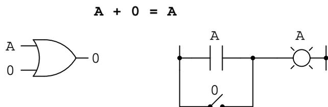
No matter what the value of  $A$ , the output will always be the same: when  $A=1$ , the output will also be 1; when  $A=0$ , the output will also be 0.
