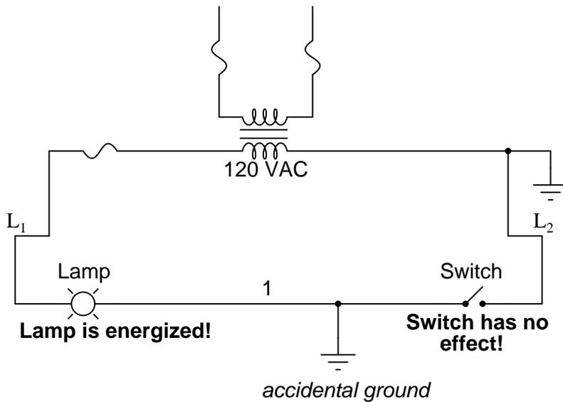
This time the accidental grounding of wire #1 will force power to the lamp while the switch will have no effect. It is much safer to have a system that blows a fuse in the event of a ground fault than to have a system that uncontrollably energizes lamps, relays, or solenoids in the event of the same fault. For this reason, the load(s) must always be located nearest the grounded power conductor in
