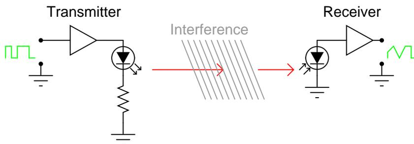
One way to avoid the problems of open-air optical data transmission is to send the light pulses down an ultra-pure glass fiber. Glass fibers will "conduct" a beam of light much as a copper wire will conduct electrons, with the advantage of completely avoiding all the associated problems of inductance, capacitance, and external interference plaguing electrical signals. Optical fibers keep the light beam contained within the fiber core by a phenomenon known as total internal reflectance.
