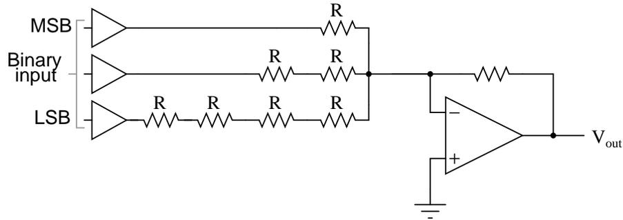
Unfortunately, this approach merely substitutes one type of complexity for another: volume of components over diversity of component values. There is, however, a more efficient design methodology.
