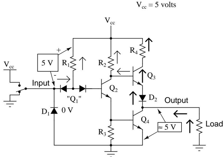
To simplify this concept, we may show the output of a gate circuit as being a double-throw switch, capable of connecting the output terminal either to  $V_{cc}$  or ground, depending on its state. For a gate outputting a "high" logic level, the combination of  $Q_3$  saturated and  $Q_4$  cutoff is analogous to a double-throw switch in the " $V_{cc}$ " position, providing a path for current through a grounded load:
