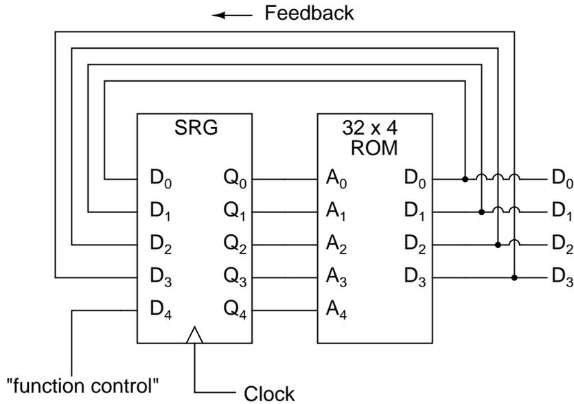
Now, just like the look-up table adder circuit that we turned into an Arithmetic Logic Unit (+, -, x, / functions) by utilizing more address lines as "function control" inputs, this FSM counter can be used to generate more than one count sequence, a different sequence programmed for the four feedback bits (A0 through A3) for each of the two function control line input combinations (A4 = 0 or 1).
